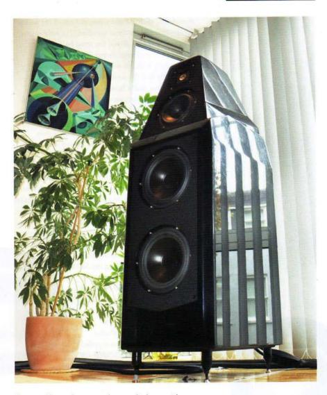
floor, and brass discs were also supplied to avoid damage. The massive head unit sits on three spikes – two at the front and one at the rear. Several different length examples of the latter are supplied, and a (hidden) look-up table on the top surface of the bass module identifies the correct spike to use for accurate time alignment according to listening distance and seated ear height.
